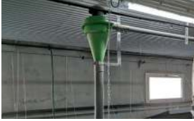
Cyclone to dispense the feed in the troughs.
